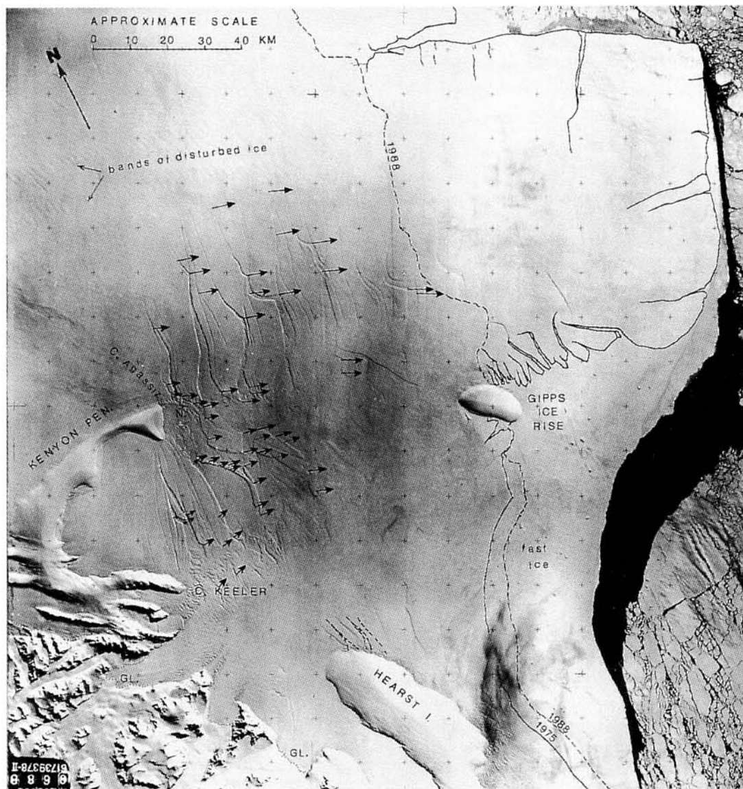
Fig. 4. KATE-200 photograph (film No. 1064; frame No. 688) of 4 October 1975, showing the chaotic region eastward of Kenyon Peninsula. The vectors indicate the surface displacement of conspicuous ice features between 1975 and 1986. The dotted lines indicate the positions of the grounding line as inferred by the change-in-slope gradient by stereoscopic observation. (Published by courtesy of SOJUZKARTA.)
